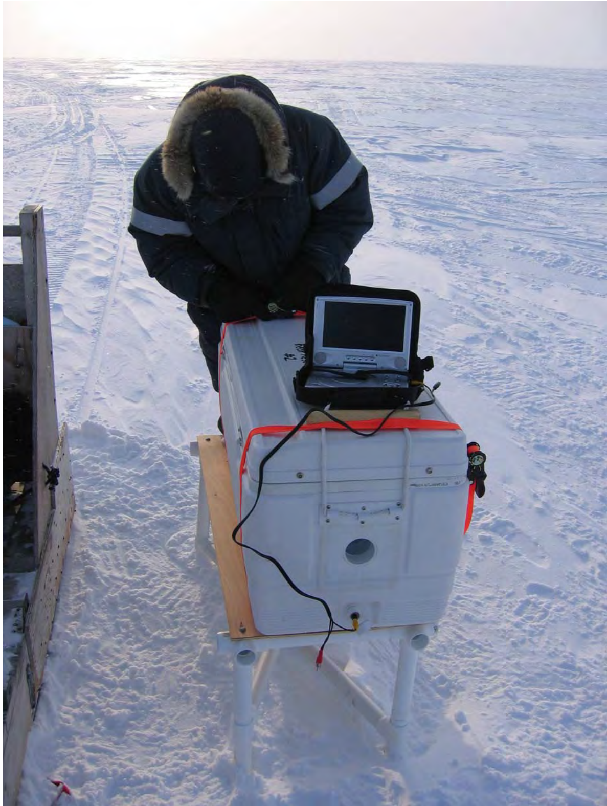
Figure 3. The self-contained camera system used for recording polar bear activity at den sites. The person is positioning the camera by observing the camera's field of view through an external monitor.
